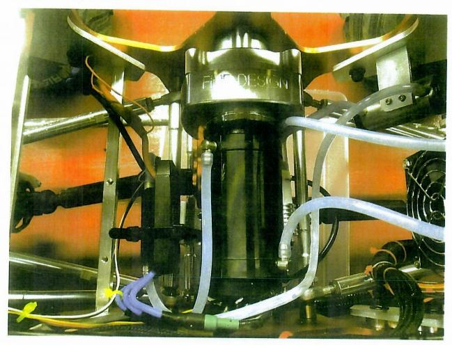
Step 7: Mounting your Hercules brushless motor, this assembly is pre-assembled to the Cutch Bell. Bolt on using existing clutch bell bolts, water flanges, facing UP.
