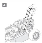
Pull the starter cord to start the engine. The engine should start within 5 pulls.
