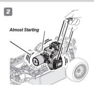
Pull start cord (about 5 times) until you hear the engine almost start, and then stop. Be careful not to flood the engine.
